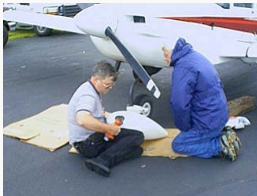
David Fletcher installs a wheel pant for a member.
